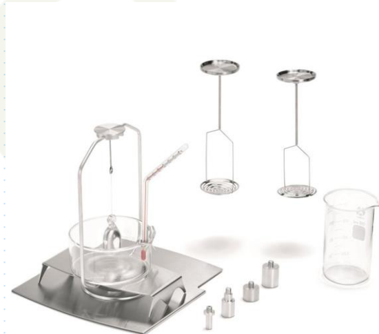
Density measurement kit
