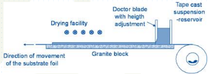
Schematic of tape casting
