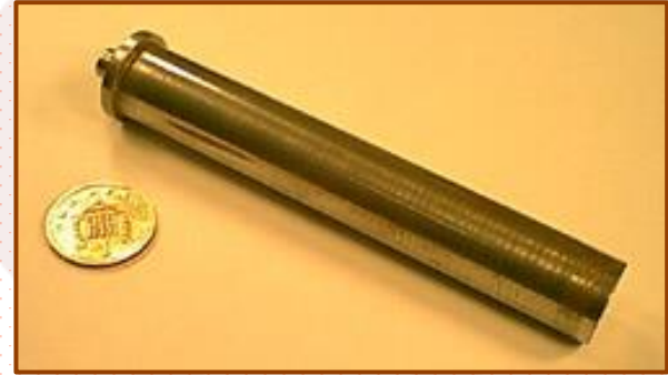
Standard Jominy end quench test specimen
